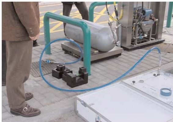
*A CNG tank involved in testing is weighed, with the prover in the foreground.*
